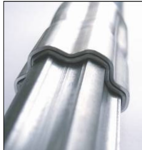
Fig 13: EMPT crimped drive shaft
