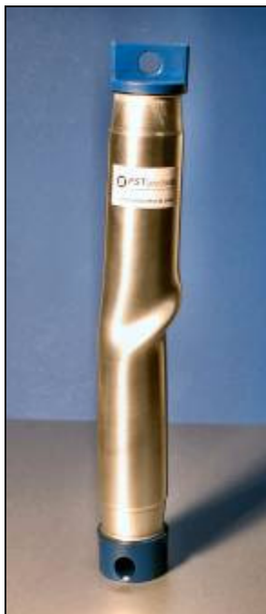
Fig 4: Successful torsion test of an EMPT welded drive shaft (aluminium tube to steel node)
