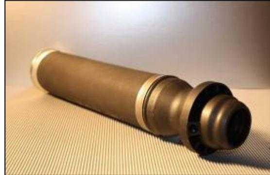
*Fig 12: EMPT crimped air suspension*
