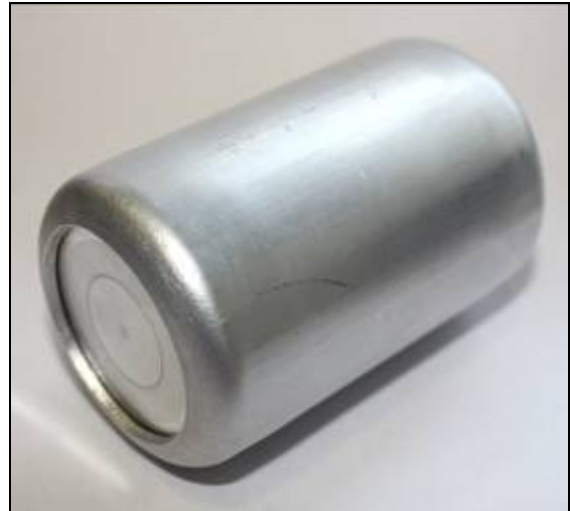
Fig 9: EMPT hemming of a pressure vessel for aluminium shock absorbers
