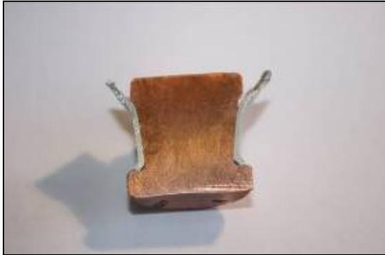
*Fig 20: EMPT welded aluminium-copper transition joint (ø25mm dia.)*
