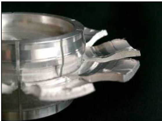
Fig 16: Successful peel test of a EMPT welded pressure vessel
