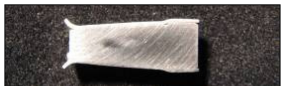
Fig 19: EMPT welding of the ferritic-martensitic steel T91 for nuclear fuel rods (ø8mm)
