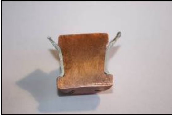
Fig 20: EMPT welded aluminium-copper transition joint (ø25mm dia.)
