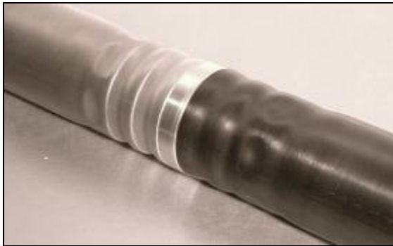
Fig 1: EMPT crimping of aluminium and steel tubes onto an aluminium node for an IP beam
