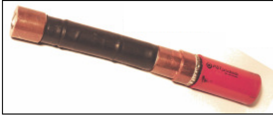
Fig 14: EMPT crimped high current cable: copper-copper and copper-steel-copper joints
