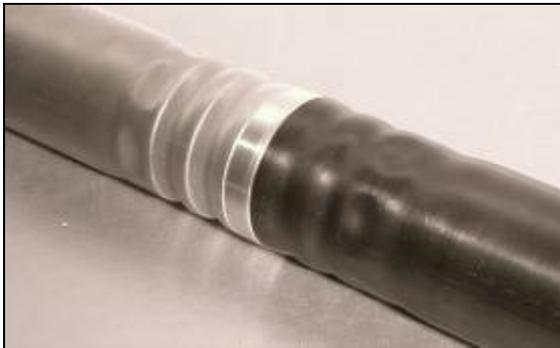
Fig 1: EMPT crimping of aluminium and steel tubes onto an aluminium node for an IP beam
