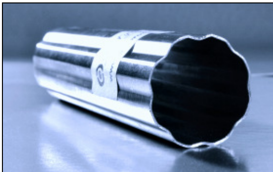
Fig 11: EMPT formed spline (ø40mm)
