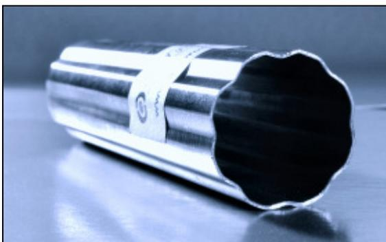
*Fig 11: EMPT formed spline (ø40mm)*
