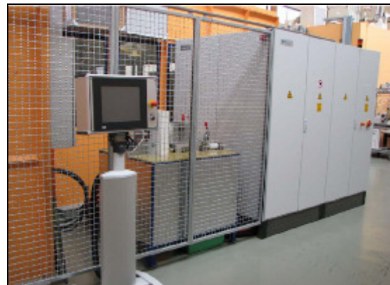
Fig 24: Heavy-duty EMPT BlueWave system PS100-10 with 100kJ energy at 10kV voltage
