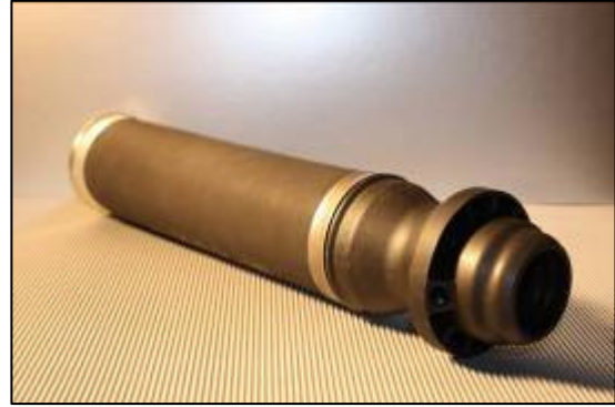
Fig 12: EMPT crimped air suspension
