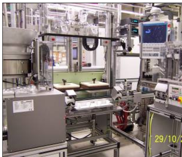
Fig. 7: PS45 EMPT crimping system of PSTproducts with a double coil concept for making two joints with one pulse in automated high-volume production at a leading German Tier 1 automotive supplier
