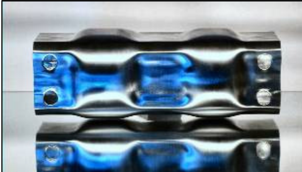
Fig. 15: Simultaneous EMPT forming and EMPT cutting of a crash box
