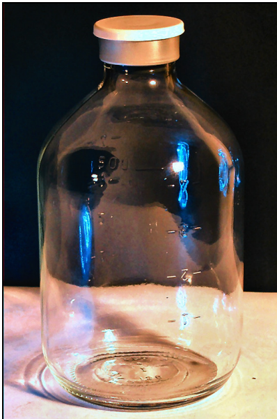
Fig. 11: EMPT crimping of a sterile aluminium lid onto a pharmaceutical glass bottle
