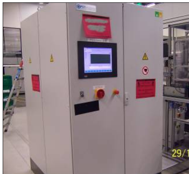
Fig. 6: PS45 EMPT pulse generator of PSTproducts at a leading German Tier 1 automotive supplier
