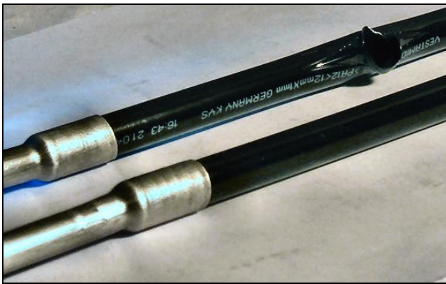
Fig. 8: EMPT crimping of steel fittings onto rubber hoses
