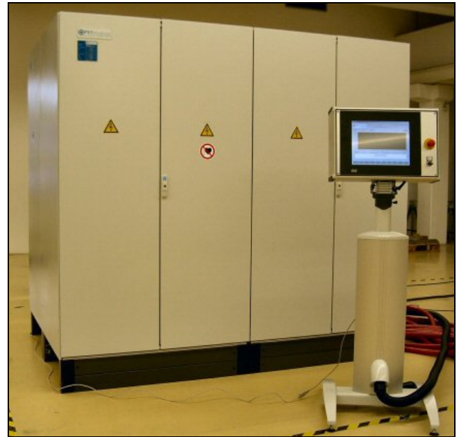
Fig. 16: A PS100 pulse generator by PSTproducts with 100 kJ power for Europe's most powerful EMPT welding machine in a leading German R&D centre
